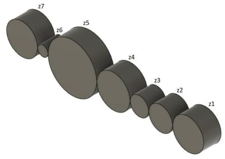
The number of teeth of the rest of gears are: z2=23, z3=18, z4=32, z5=47, z6=10, z7=30. Calculate the RPM of the final gear z7. (answer format round to nearest decimal eg:12.34) Correct answer: **3600.00 rpm**
